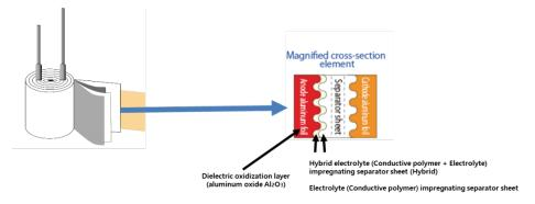
Since 2019, Samwha Electric has been supplying conductive polymer hybrid and "YM" series, provided in voltage range from 25V to 63V with capacitance of 47 to 680µF, will expand the market further into 5G.
