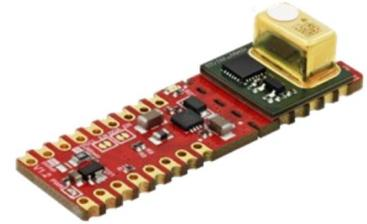
Testing IoT system behavior with an integrated prototyping concept from Infineon (Easy mix and match approach, sensor, security, microcontroller and adapter boards).
