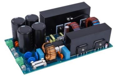
The EVAL-PFC5KIKWWR6SYS is an evaluation board for Aircon and EV charger applications. It features the TRENCHSTOP™ 5 WR6 (IKWH40N65WR6), EiceDRIVER™ Gate driver IC (1ED44175N01B) as well as a rapid diode (IDW60C65D1).
