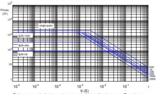
Pulse on a regular basis; maximum permissible peak pulse power (P-max) as a function of pulse duration  $(t_i)$ .
