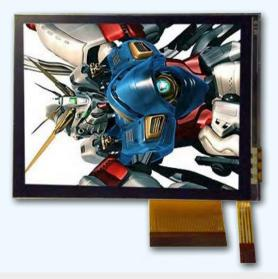
Because OLEDs do not require backlighting, they consume much less power than LCDs. This is especially important for batteryoperated devices such as cell phones.
