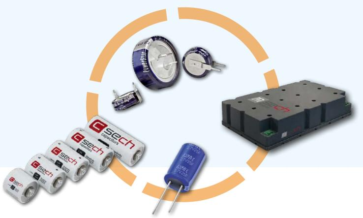
The key point of this technology is the special electrode with its surface coated with activated carbon. The porous structure of this coating expands the surface significantly and allows a capacity up to thousands of Farad. The Electric Double Layer Capacitor does not have a typical dielectric rather it uses the electrolyte solution as a function of the dielectric.
