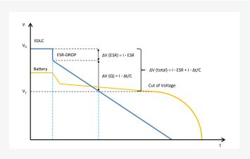
The ESR-Drop (DIR) shown on the graph above is a voltage drop caused by the ultracapacitor's Equivalent Series Resistance (ESR) and is directly proportional to the capacitor's ESR. Especially in cases of high discharge currents the voltage drop can be important and thus should be calculated.
