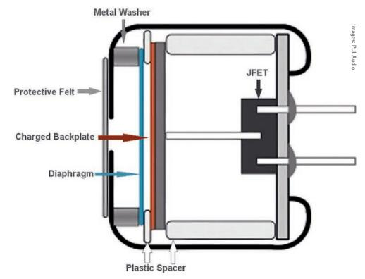
Figure 1: Schematic diagram of an electret condenser microphone
