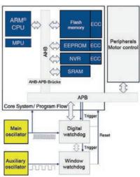
Figure 3: A window watchdog and a digital watchdog monitor the system clock and program execution of the motor controllers.
