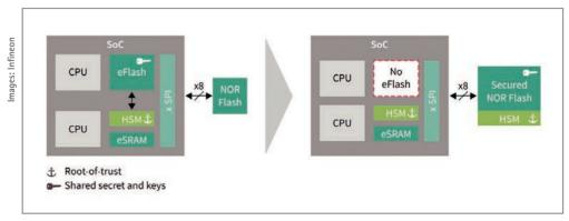
Figure 1: De-integration of embedded flash (eFlash) from the SoC.
