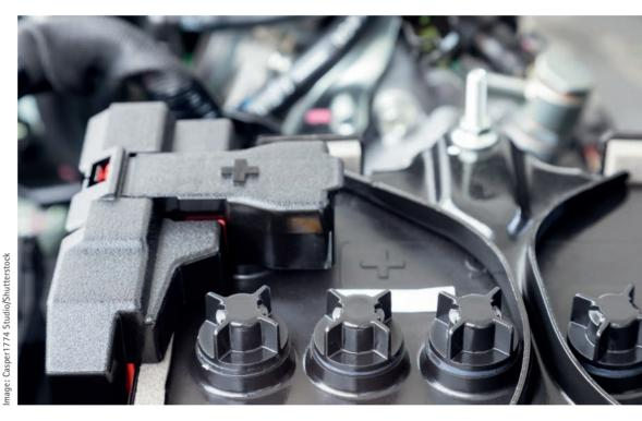
arameters such as battery current and voltage are measured to monitor the battery in the vehicle. The electronics use these parameters to calculate the residual energy stored in the battery, among other variables. Based on this, a control unit can decide which loads may be switched on or must be switched off to ensure that vital assistance functions remain available.
