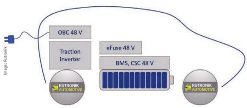
The electronic power applications in an LSEV
