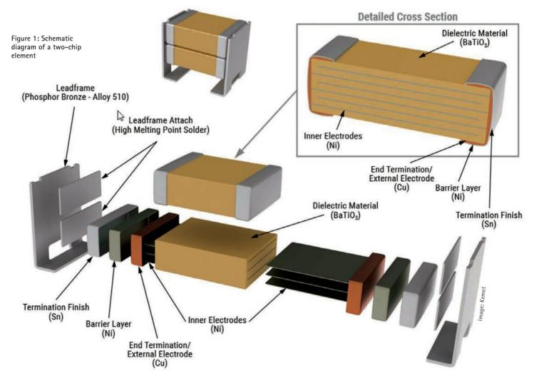
Figure 3: The leadframe gives the MLCC greater robustness against thermal and mechanical stresses.
