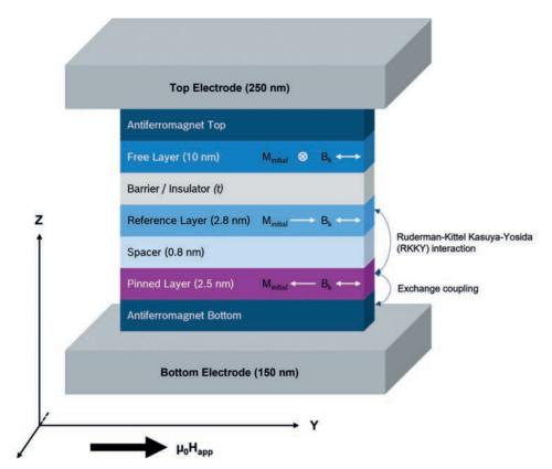
Figure 3: Schematic diagram of an MTJ stack and orientation of simulation input vectors relative to coordinate
