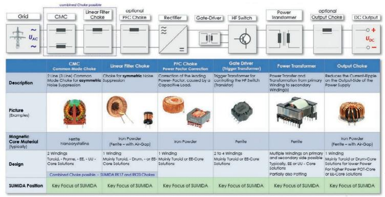
Figure 1: Sumida covers all inductors for switched-mode power supplies and partially and fully implements application-specific components.
