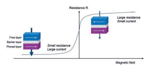
Figure 2: The TMR effect: If the magnetization directions of the free layer and the pinned layer run parallel, the resistance is low and a large current flows (left). If they run in opposite directions, the resistance is high and only a weak current flows (right).
