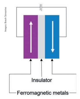
Figure 1: Schematic TMR arrangement with two ferromagnetic layers and an intermediate insulating layer
