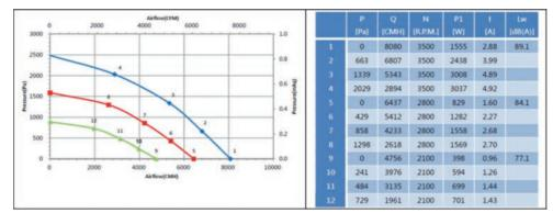
Figure 2: Suppliers usually specify several characteristic curves for their fans for operation at different speeds.
