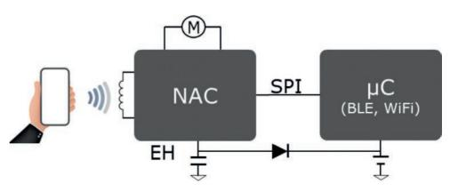
Using an SPI interface, the NAC1080 can communicate with external devices.
