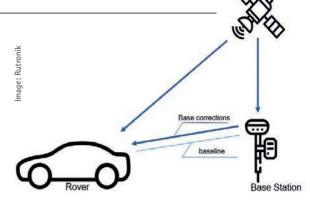
Two GNSS receivers communicate via a base station to determine a position accurately.
