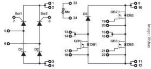
The components in Vishay's VS-ENM040M60P power module
