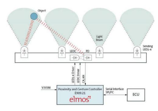
Figure 2: Using Halios technology, the E909.21 controller from Elmos Semiconductor achieves high sensitivity as well as immunity to ambient light and rapid changes in brightness.
