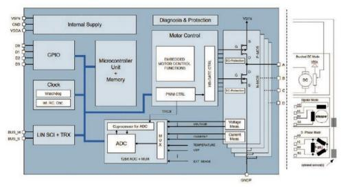
Figure 3: The E523.63 is an all-in-one chip for low to medium power actuator and fan applications.
