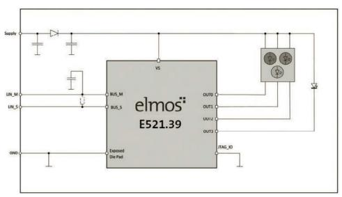
Figure 1: The E521.39 RGBW LED driver from Elmos Semiconductor features an integrated microcontroller and LIN transceiver, four PWM generators, and four current sources, as well as diagnostic capabilities.
