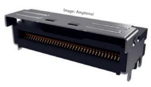
Figure 4: Amphenol's durable Mini Cool Edge IO (MCIO) plug connector can transmit high-speed signals of up to 64 Gbit/s over a distance of 1 m and meets new PCIe Gen6 requirements.
