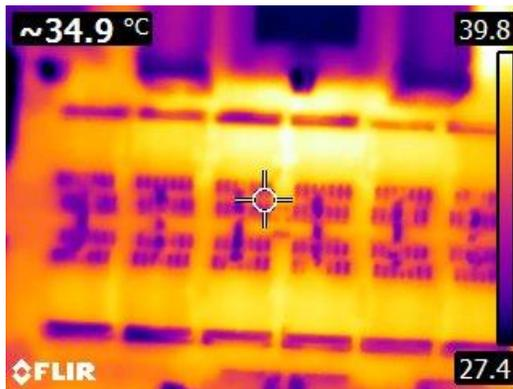
Figure 23: Stress Test with 30 A
