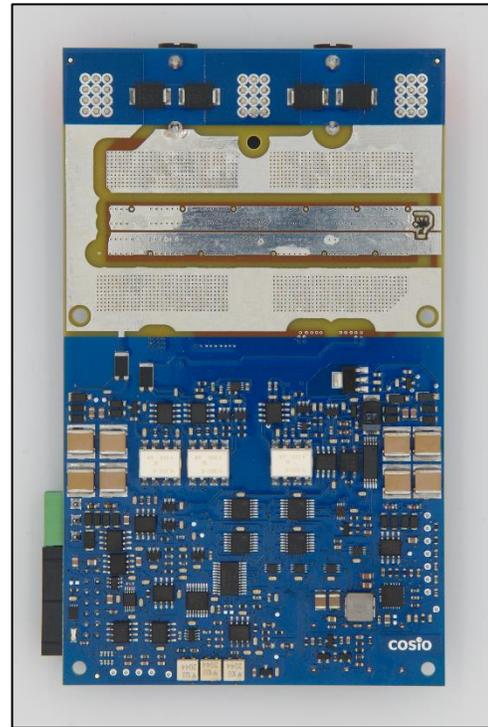
Figure 2: Vishay eFuse 800 VDC 50 A (Bottom View)
