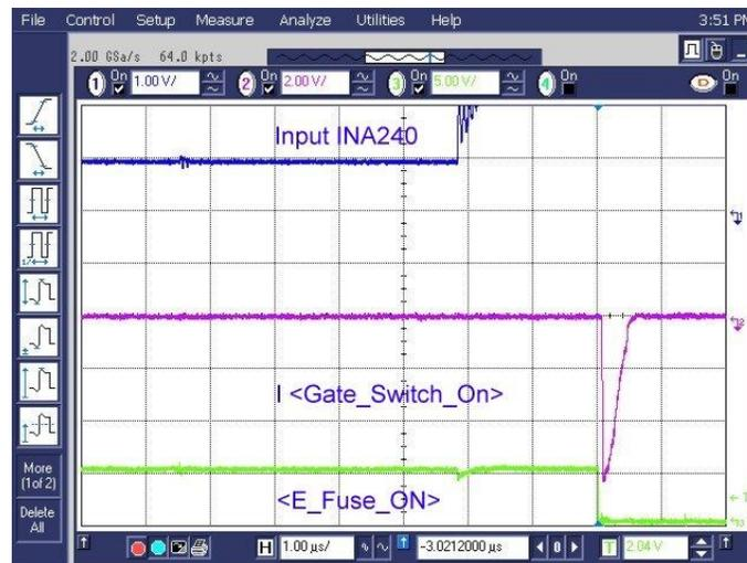
Figure 18: Switching Off after a Short Circuit Event
