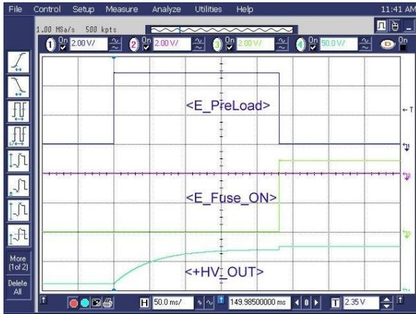
Figure 11: Successful Switch-On Procedure, First Preload Stage
