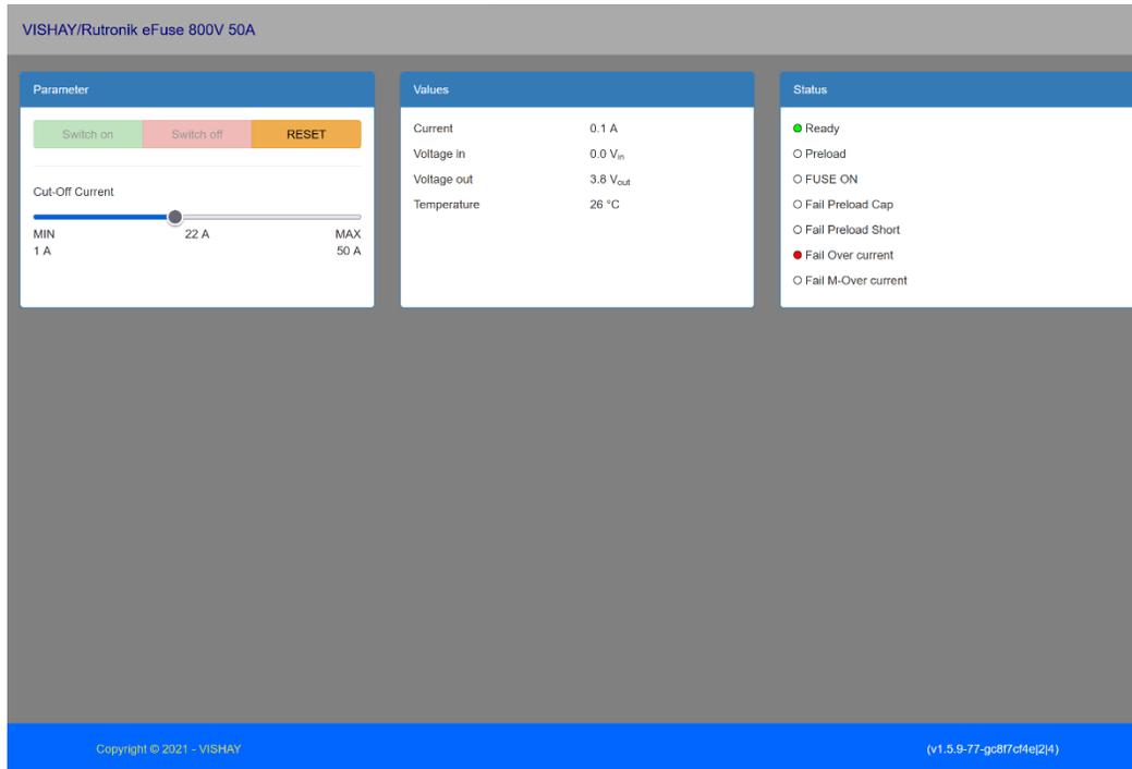
Figure 30: Web Interface after an error occurred
