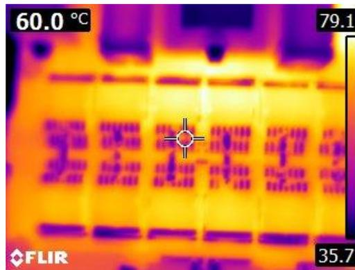
Figure 25: Stress Test with 50 A (60min)
