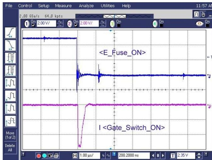
Figure 17: Switch-Off Procedure of the eFuse
