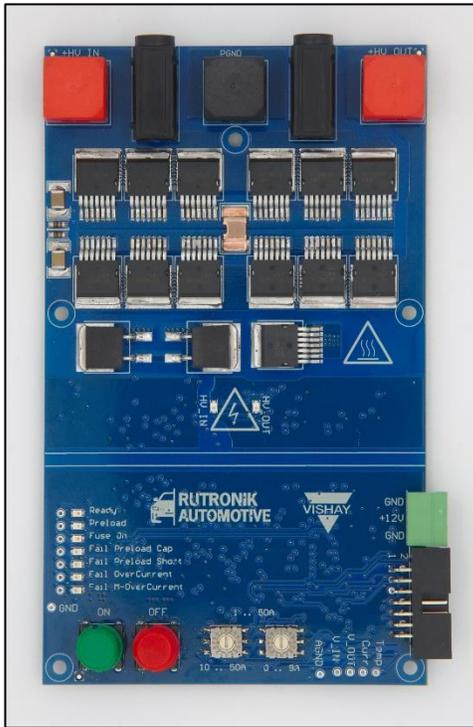
Figure 1: Vishay eFuse 800 VDC 50 A (Top View)
