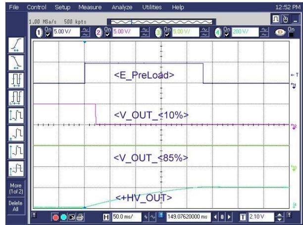
Figure 14: Switch-On Procedure Aborts During the Second Preload
