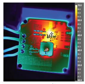
T<sub>ambient</sub> = 30 °C Highest Temp at 168 W = 66 °C
