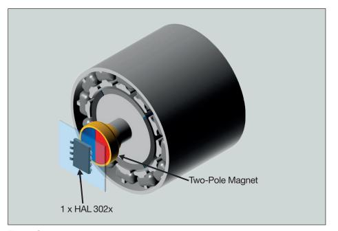
Fig. 1: Sensor application setup
