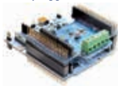
Expansion board plugged on the Nucleo board
