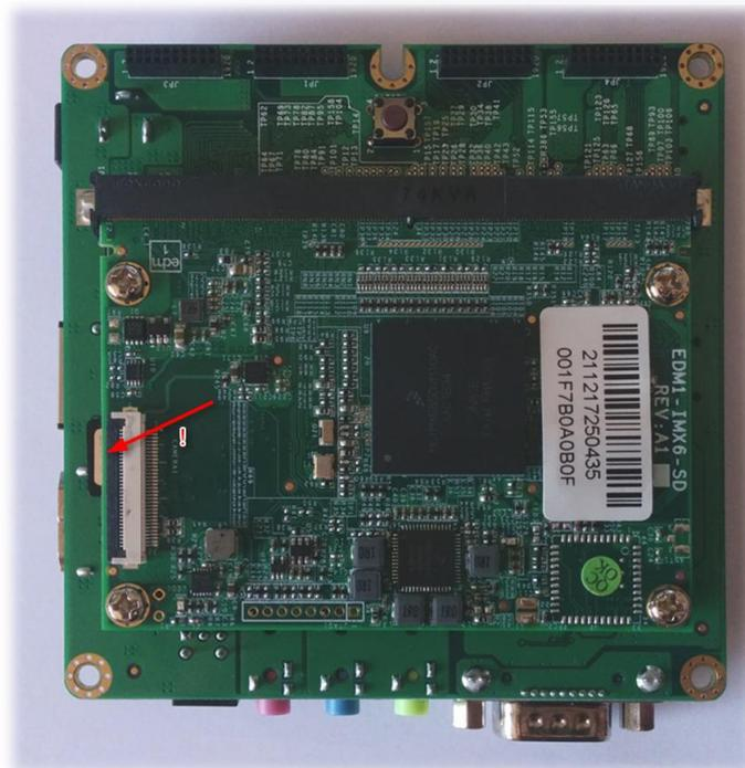
If the  $\mu$ SD card needs to be changed, gently press the connector and the  $\mu$ SD card will spring out.
