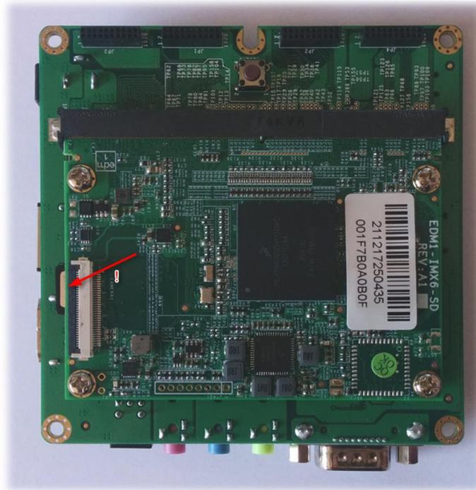
In order to replace the  $\mu$ SD card gently press the connector and the  $\mu$ SD card will spring out.
