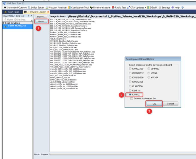
2. Select the controller **KW41Z** (2), which is used on PAN4620 device.
