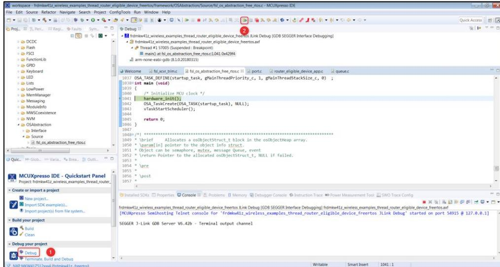
➔ The software will be flashed with the onboard **J-Link-OB-SAM3U128** to the PAN4620 module. Wait till this process is finished.
