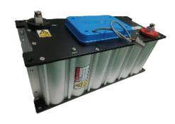
This new series of electrochemical, double-layer, series-connected SuperCapacitor modules offers excellent pulse power handling characteristics based on the combination of very high capacitance and very low ESR. Used by themselves or in conjunction with primary or secondary batteries, they provide extended back up time, longer battery life, and provide instantaneous power pulses as needed. Offers great solutions to Hold Up, Energy Harvesting, and Pulse Power Applications.
