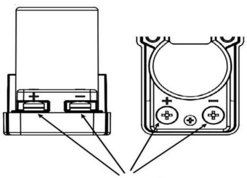
Terminal screws: M4 Maximum torque: 2 Nm
