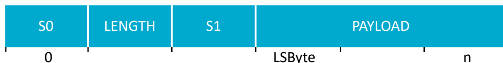
Figure 108: Representation of a RADIO packet in RAM
