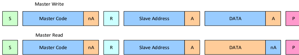
Figure 3-101 I2C Write Frame Format in HS Mode
