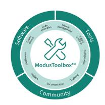
Run-time software, comprised of middleware, device drivers, and code examples, is provided via an extensive collection of GitHub-hosted repositories usable directly within the ModusToolbox™ desktop applications. Additional details are available from the ModusToolbox™ software repository overview.
