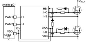
\* With digital controller (VDD=3.3V), the driver VDD is taken out of aux
