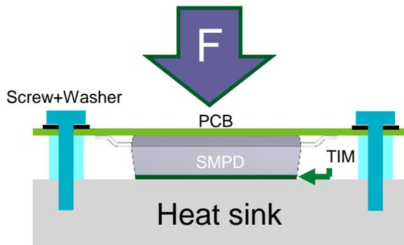
Correlation of mounting force  $F$  and thermal resistance  $R_{thch}=f(F,t)$
