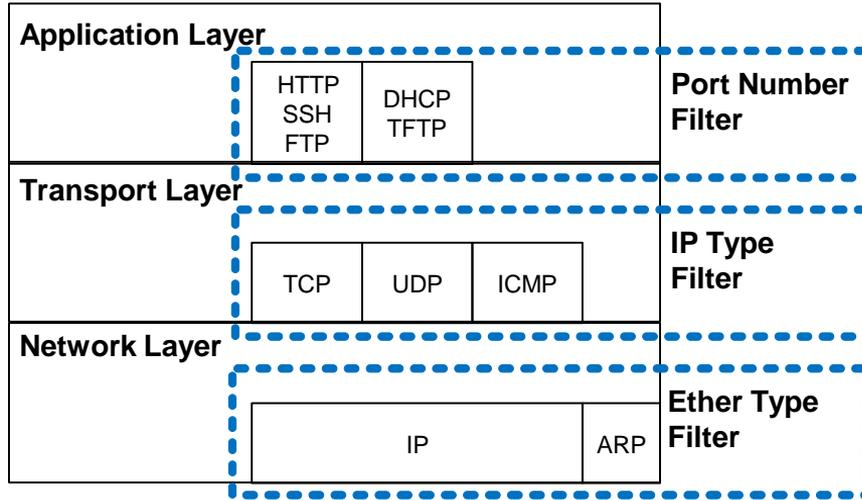
Offload with discard filter for Ping packets
