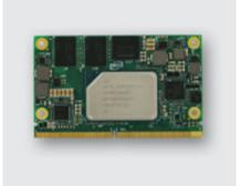
SMARC® Rel. 2.1.1 Computer on Module (CoM) with Intel® Atom® x6000E Series and Intel® Pentium® and Celeron® N and J Series (Codename: Elkhart Lake) Processors for FuSa applications. (formerly HALLEY - C93)
