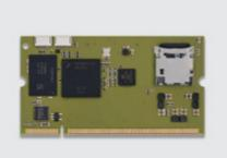
SODIMM-200 CPU Computer on Module (CoM) with NXP i.MX 8M Mini Applications Processors. (formerly Trizeps VIII Mini)
