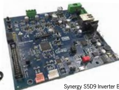
Synergy S5D9 Inverter Board Max. 48 V DC , 5 A max
