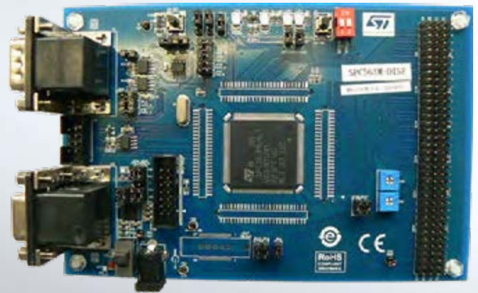
Discovery+ Kit for SPC56 M line with SPC563M64L. Order code: SPC563M-DISP
