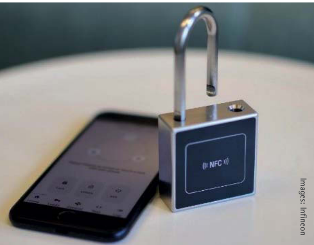
The NAC1080 can be used as a motor driver for battery-free padlocks.
