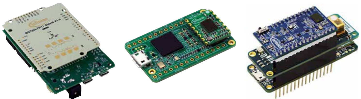
Figure 3: Development kits complement the radars: 24 GHz demo Distance2GoL (left), demo BGT60TR13C MMIC (center), and 60 GHz connected sensor kit (right).
