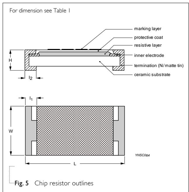
Fig. 5 Chip resistor outlines
