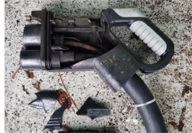
Figure 4. Exploded connector, Daegu, South Korea, 2018. The explosion was allegedly caused by a short-circuit [7].
