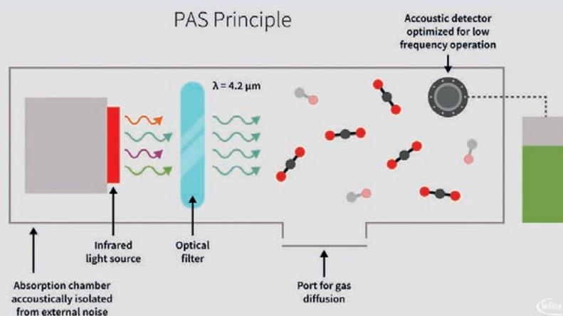
Photoacoustic spectroscopy to determine the concentration of CO<sub>2</sub>
