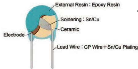
Figure 3: Structure of a radial single-layer capacitor
