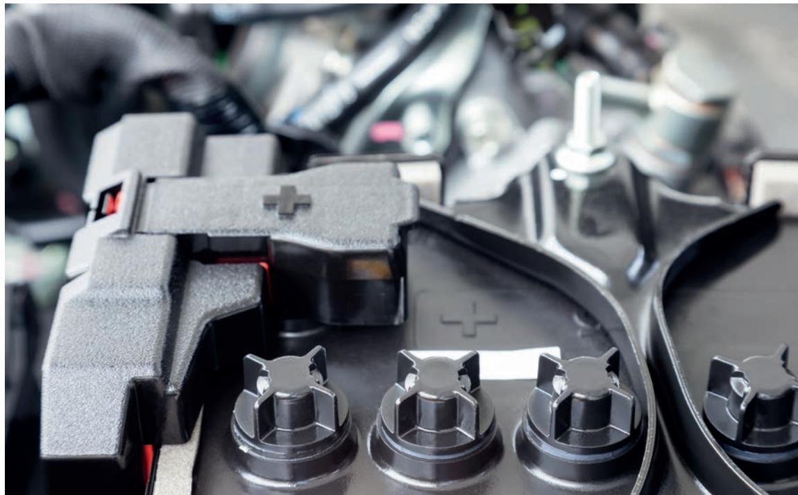
**P**arameters such as battery current and voltage are measured to monitor the battery in the vehicle. The electronics use these parameters to calculate the residual energy stored in the battery, among other variables. Based on this, a control unit can decide which loads may be switched on or must be switched off to ensure that vital assistance functions remain available.
