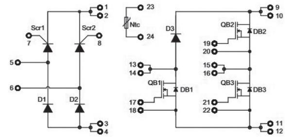
The components in Vishay's VS-ENM040M60P power module
