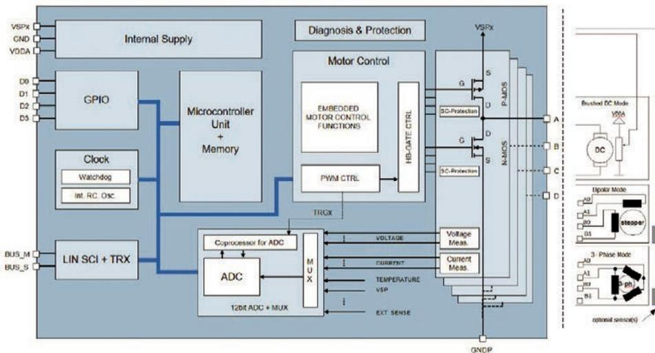
vanced control algorithms such as field-oriented control (FOC) with low CPU load. Both the E523.63 and the E533.06 are AEC-Q100 qualified and comply with the ISO 26262 standard (ASIL B). Their broad temperature range extends from  $-40^{\circ}\text{C}$  to  $+150^{\circ}\text{C}$ .
