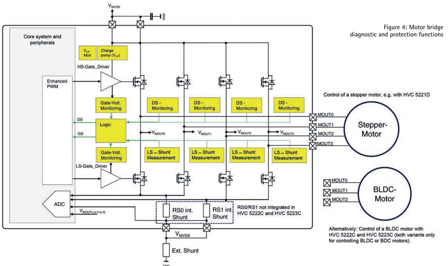
Figure 4: Motor bridge diagnostic and protection functions
