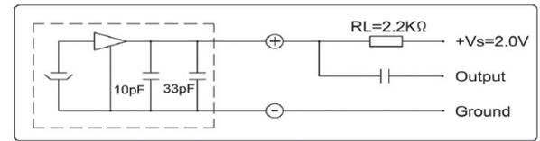
Figure 2: Amplifier circuit of an electret condenser microphone
