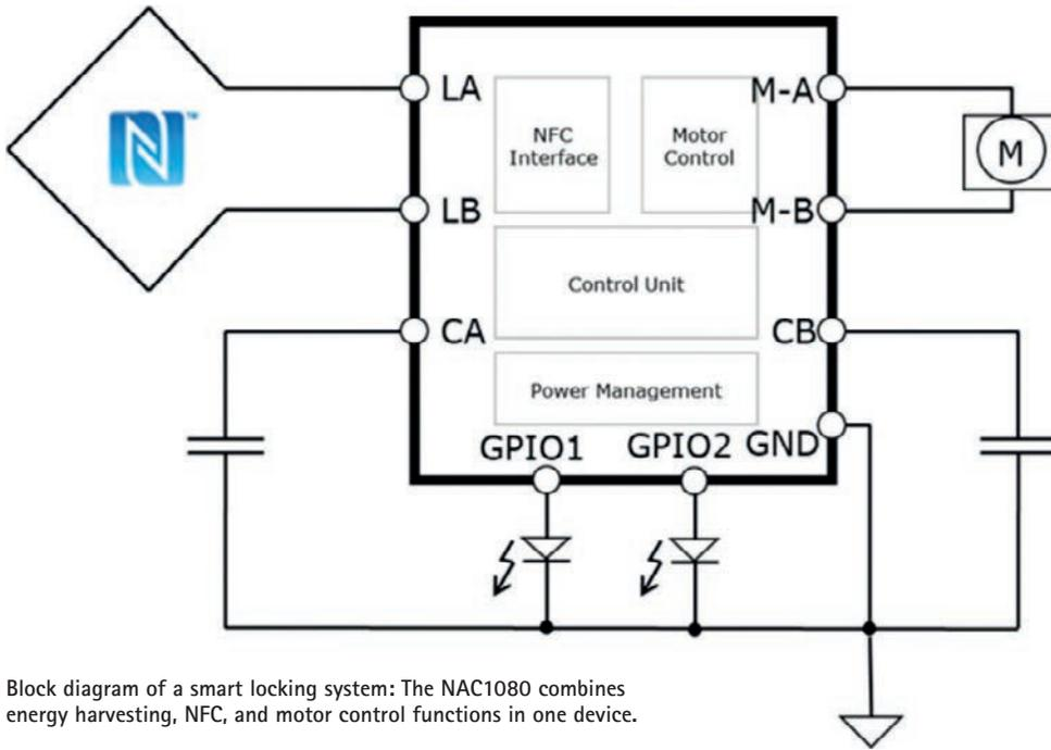
Block diagram of a smart locking system: The NAC1080 combines energy harvesting, NFC, and motor control functions in one device.
