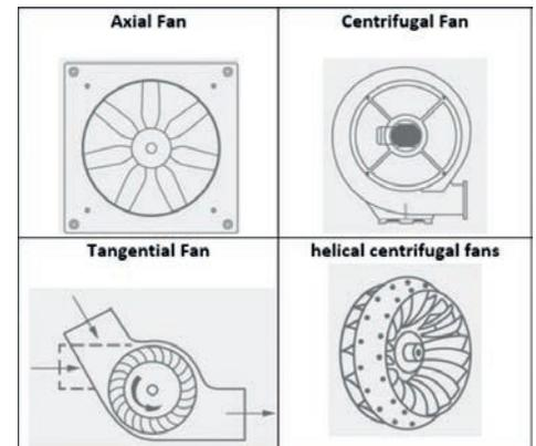
Figure 1: Fan types by direction of airflow
