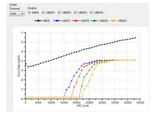
High Temperature Data Retention Testing: UBER after P/E cycling
