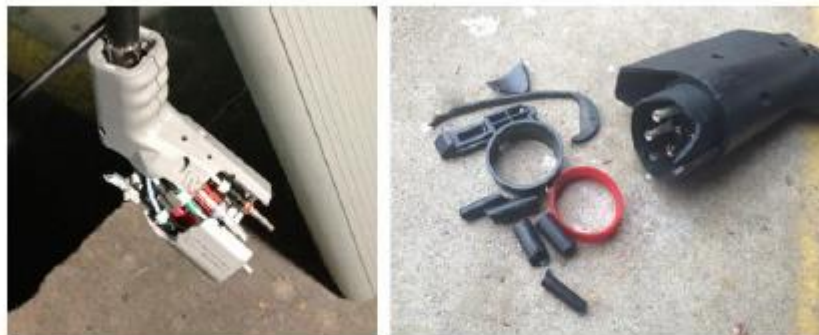
Figure 2. Common mechanical failures of connectors, including damage to the housing (left [3]), damage to the mating interface (right [4])
