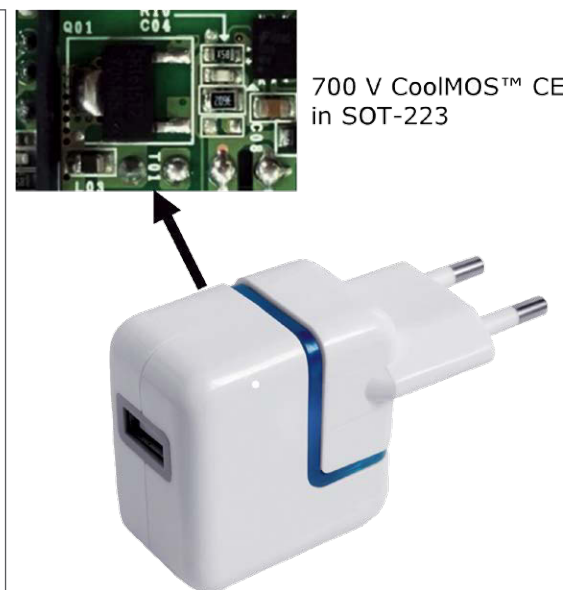
Figure 3: Thermal evaluation was conducted on an 18 W mobile phone charger as shown.
