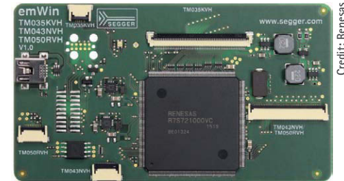
Rutronik offers a system solution with RZ/A1H and Tianma TFT screen with Segger emWin. The kit is immediately available from stock.
