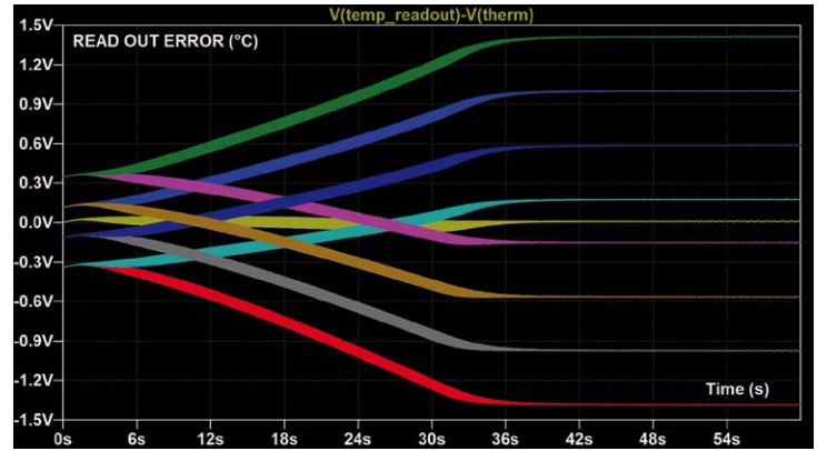
Figure 5: Temperature measurement uncertainty with dR25 = \pm 1\% and dB = \pm 0.5\% for the NTC and \pm 0.5\% for the fixed resistor.
