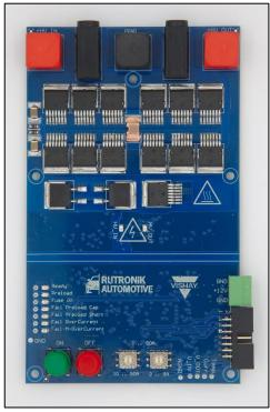
Figure 1: Vishay eFuse 800 VDC 50 A (Top View)
