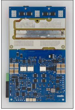
Figure 2: Vishay eFuse 800 VDC 50 A (Bottom View)
