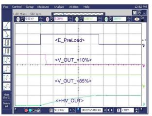
Figure 14: Switch-On Procedure Aborts During the Second Preload
