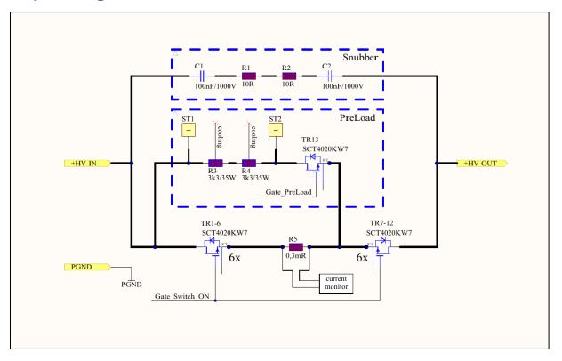
Figure 3: Overview of the High Voltage Side
