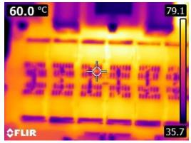
Figure 25: Stress Test with 50 A (60min)
