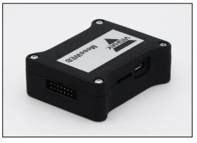
Figure 28: Shrouded Connector and Slot for the SD Card
