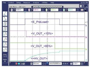
Figure 13: Successful Switch-On Procedure, Second Preload
