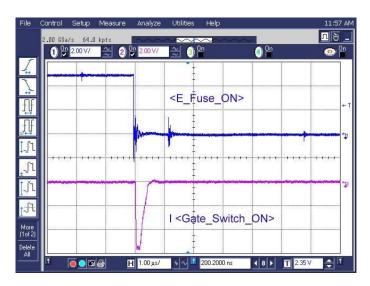
Figure 17: Switch-Off Procedure of the eFuse
