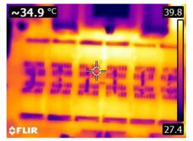
Figure 23: Stress Test with 30 A
