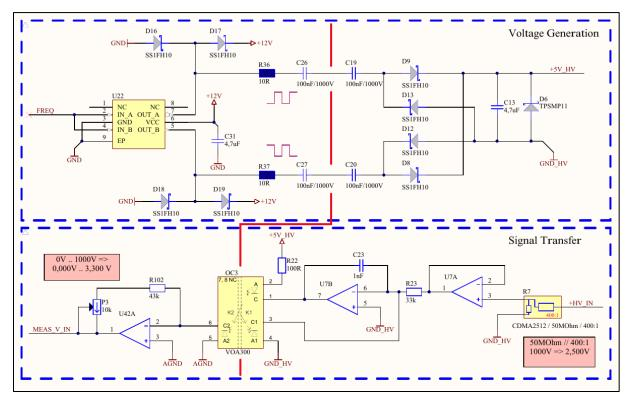
Figure 4: Connections between High Voltage and Control Side
