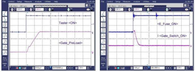
Figure 15: Switching on the Preload MOSFET
