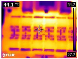
Figure 24: Stress Test with 40 A (20min)
