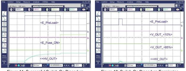
Figure 11: Successful Switch-On Procedure, First Preload Stage
