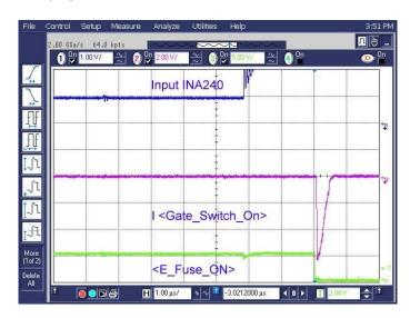
Figure 18: Switching Off after a Short Circuit Event
