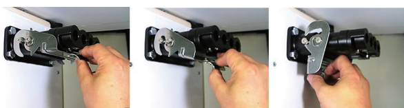
JK11 disengagement operation (Pinch the lock while pushing the lever down to disengage)
