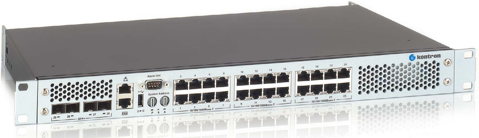
With the RES2404-PTP, Kontron is offering a managed 19" high-performance switch for industrial use with up to 24 10/100/1000BASE-T ports and four 10G-SFP+ ports for copper or fiberglass lines, a wider temperature range of -25°C to +70°C, and Power-over Ethernet functionality.
