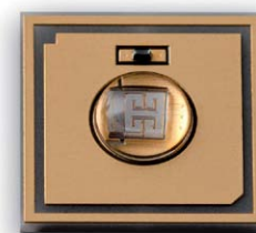
Figure 2: High output—the high-power UVC LED from Bolb with 100 mW at 250 mA, with and without mount
