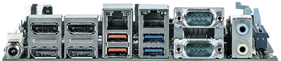
The skyline of the new D3713-V/R Mini-ITX motherboards from Kontron with AMD Ryzen Embedded V1000/R1000 processors is densely packed with many interfaces covering almost the entire breadth of the form factor.
