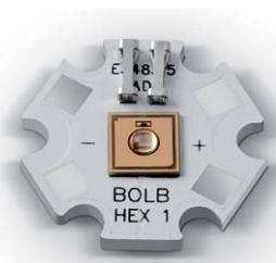
Figure 2: High output—the high-power UVC LED from Bolb with 100 mW at 250 mA, with and without mount
