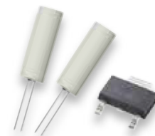
Ceramic housed & SOT housed sensor
